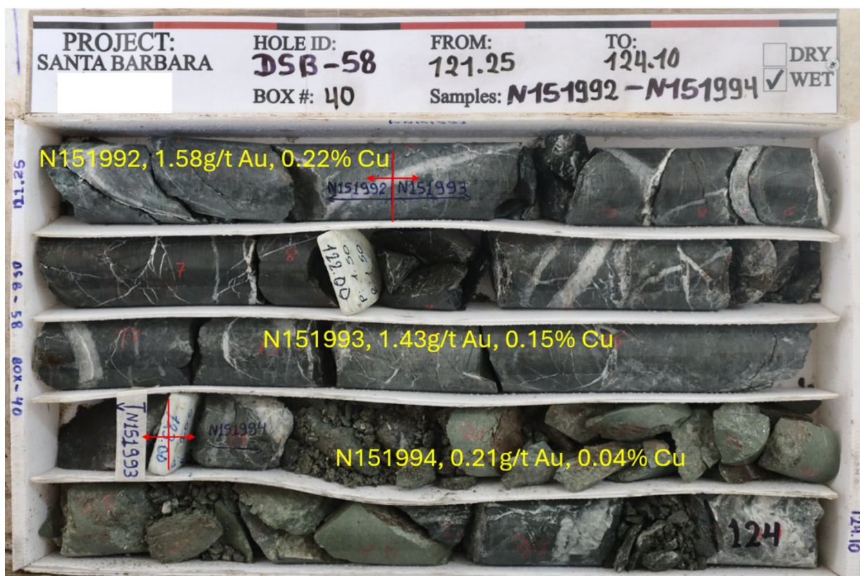
Figure 5: Core photo of DSB-58, Box 40, from 114.10 to 121.25m, mineralized basaltic andesite with quartz veining. Note that the sample N151994 contains a 0.7m wide post-mineralization grayish green andesite dyke, accordingly the grades of gold and copper of the sample are diluted.
