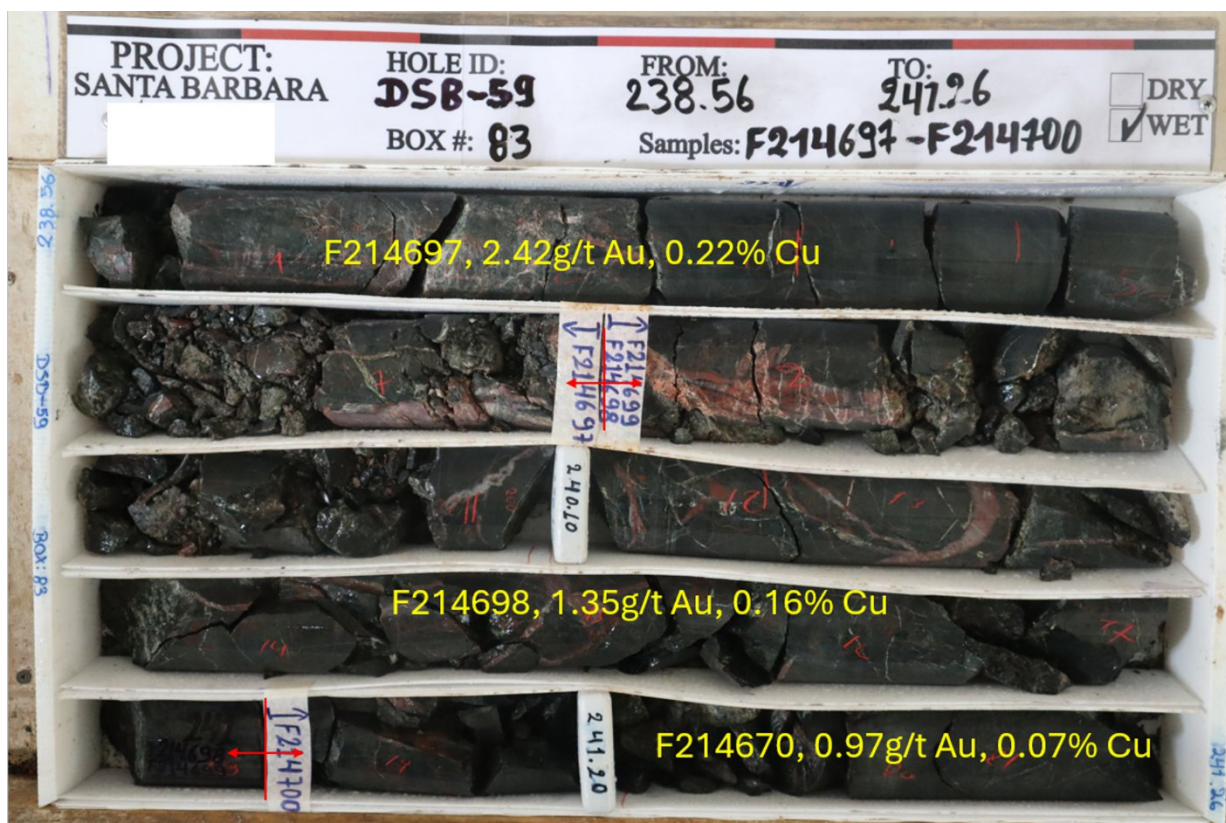
Figure 7: Core photo of DSB-59, Box 83, from 238.56m to 241.26m, mineralized basaltic andesite cut by quartz-hematite veining.
