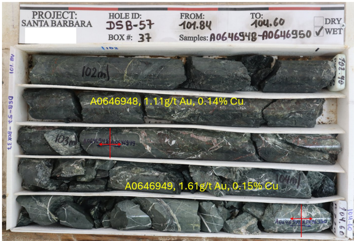
Figure 3: Core photo of DSB-57, Box 37, from 101.84m to 104.96m, mineralized basaltic andesite cut by quartz-hematite veining overprint by post-mineralization calcite veining.
