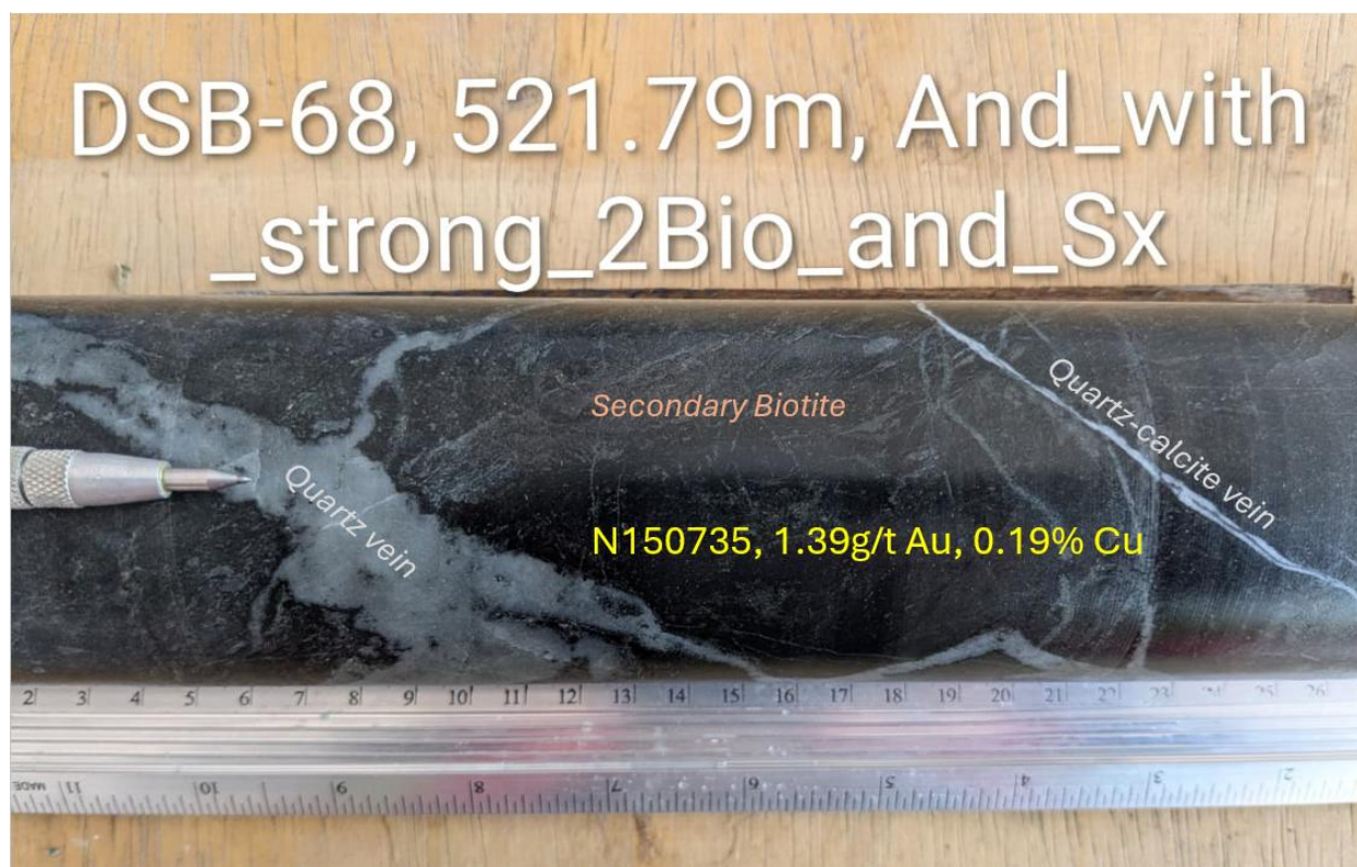
Figure 5: Core photo of DSB-68, depth 521.79m, mineralized basaltic andesite cut by quartz and quartz-calcite veining, with patchy dark brownish secondary biotite (potassic alteration) and dissemination of pyrite and chalcopyrite.
