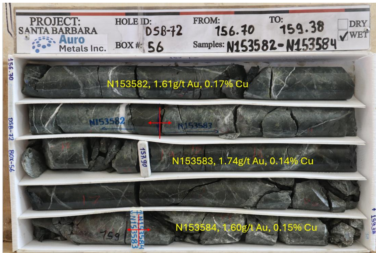
Figure 5: Core photo of DSB-72, Box 56, from 156.7m to 159.38m, mineralized volcano-sediments cut by quartz veining.
