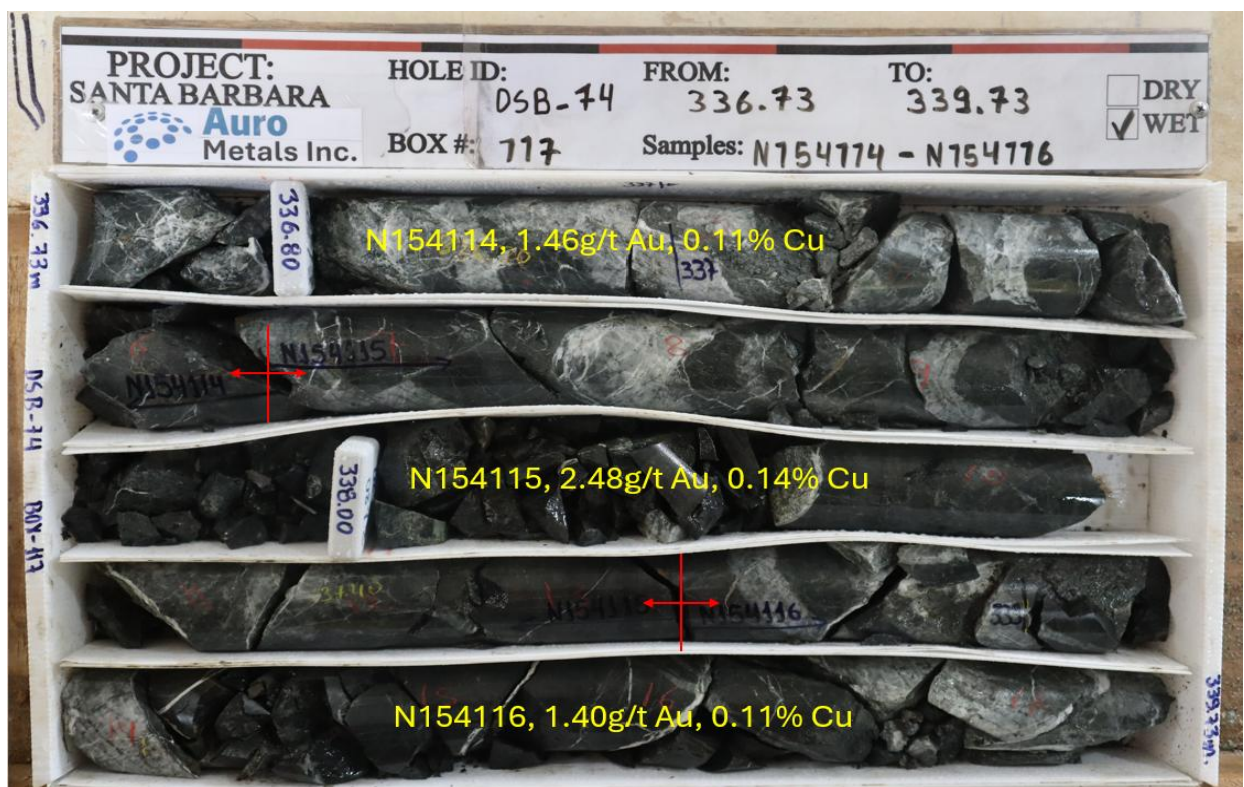
Figure 8: Core photo of DSB-74, Box 117, from 336.73m to 339.73m, mineralized basaltic andesite cut by quartz veining.
