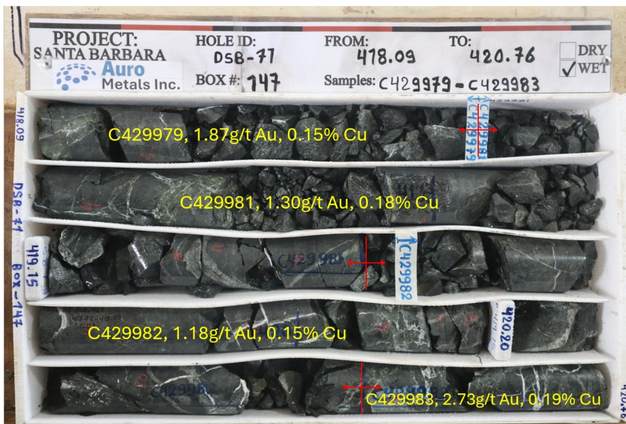
Figure 3: Core photo of DSB-71, Box 147, from 418.09m to 420.76m, mineralized basaltic andesite cut by quartz veining.
