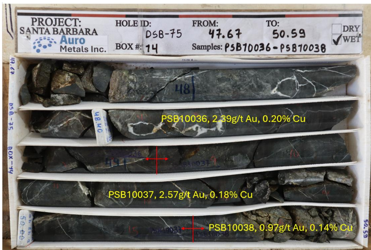
Figure 10: Core photo of DSB-75, Box 14, from 47.67m to 50.59m, mineralized diorite porphyry cut by quartz veining.
