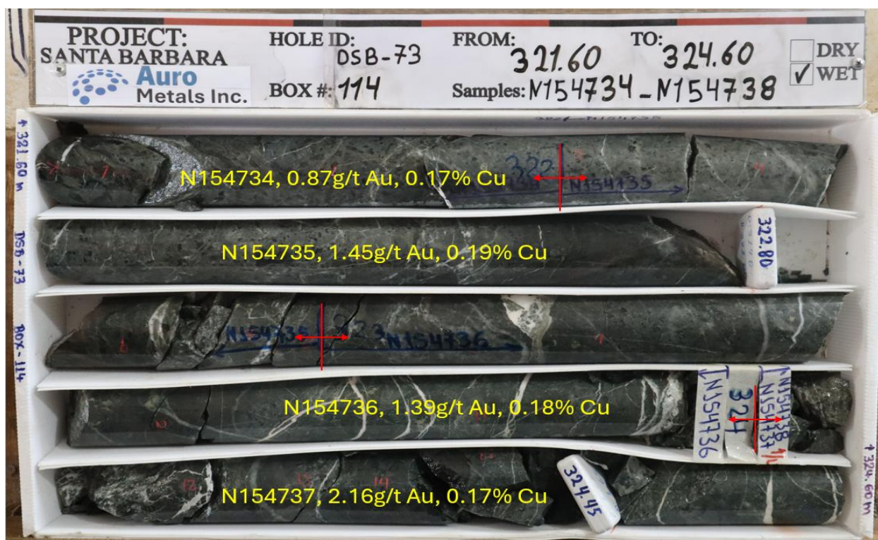
Figure 7: Core photo of DSB-73, Box 114, from 321.6m to 324.6m, mineralized diorite porphyry cut by quartz veining.
